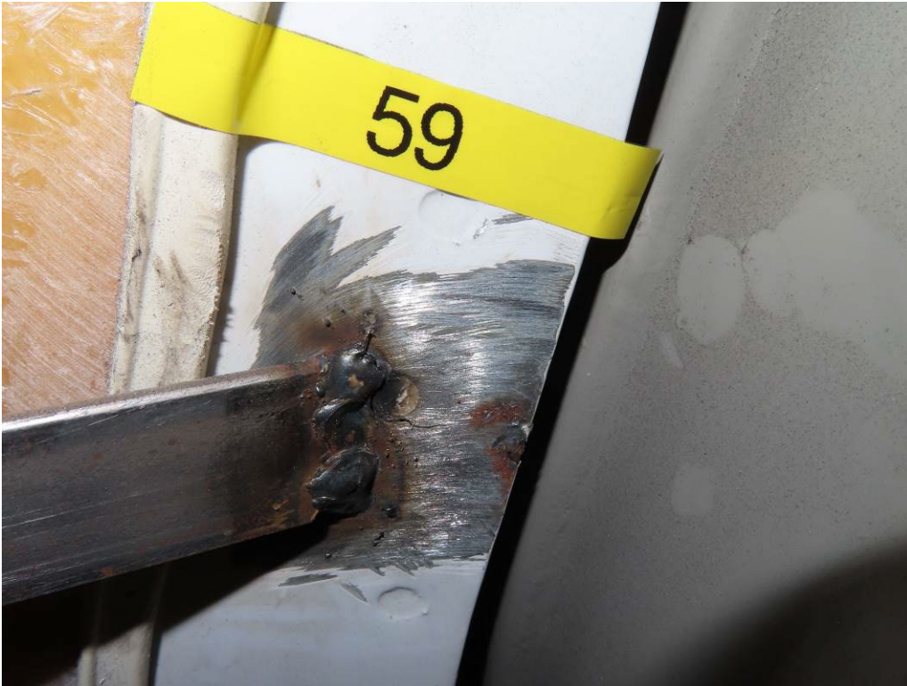
CRACK #59 – STEEL STRAP THAT WAS ADDED TO BODY BEHIND DRIVER HAS CRAKED (7,486 TEST MILES)
