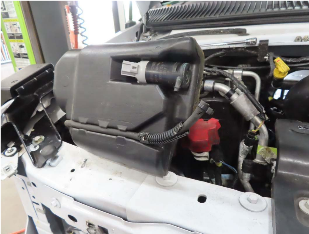
DAMAGED HOSE ON WASHER TANK (7,486 TEST MILES)
