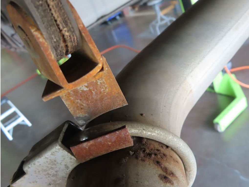
EXHAUST HANGER ON STREETSIDE HAS CRACKED AND SEPARATED (5,533 TEST MILES)
