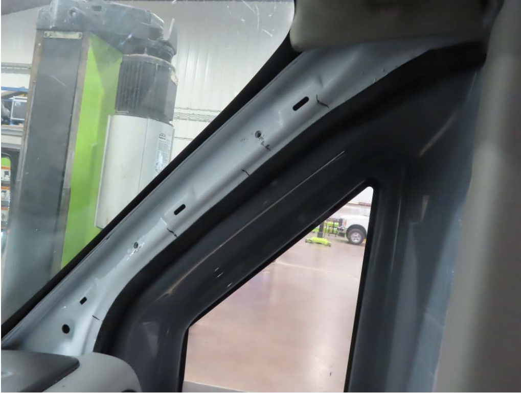
SCREWS THAT HOLD THE OUTER PANEL ON THE SUPPORT POST ADJACENT TO THE WINDSHIELD ON THE CURBSIDE ARE BROKEN (1,123 TEST MILES)
