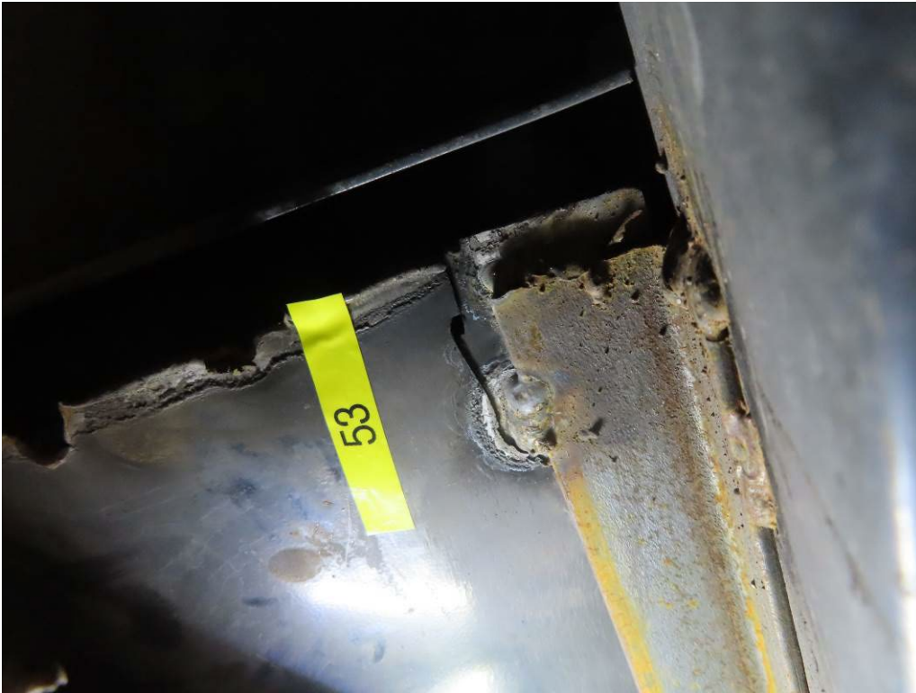
CRACK #53 – CRACK IN REAR HEATSHIELD ABOVE HORIZONTAL CROSSMEMBER (7,486 TEST MILES)
