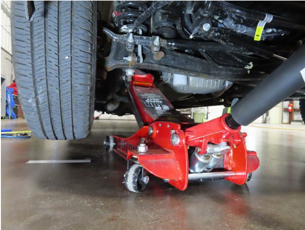
JACK IN PLACE – FRONT
