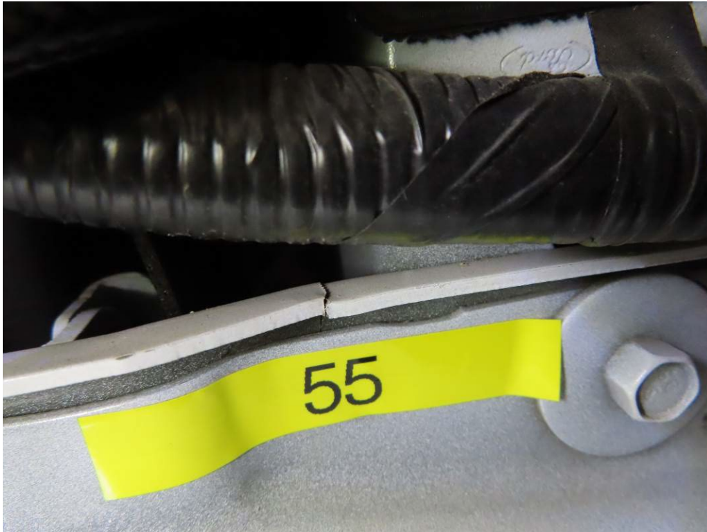
CRACK #55 – CRACK IN BODY BEHIND GRILLE IN FRONT OF THE A/C CONDENSER (7,486 TEST MILES)
