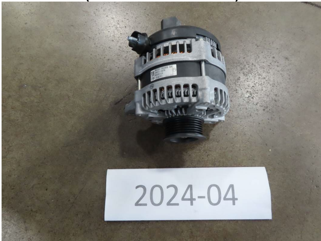
ALTERNATOR REMOVAL AND REPLACEMENT (0.50 LABOR HOURS)
