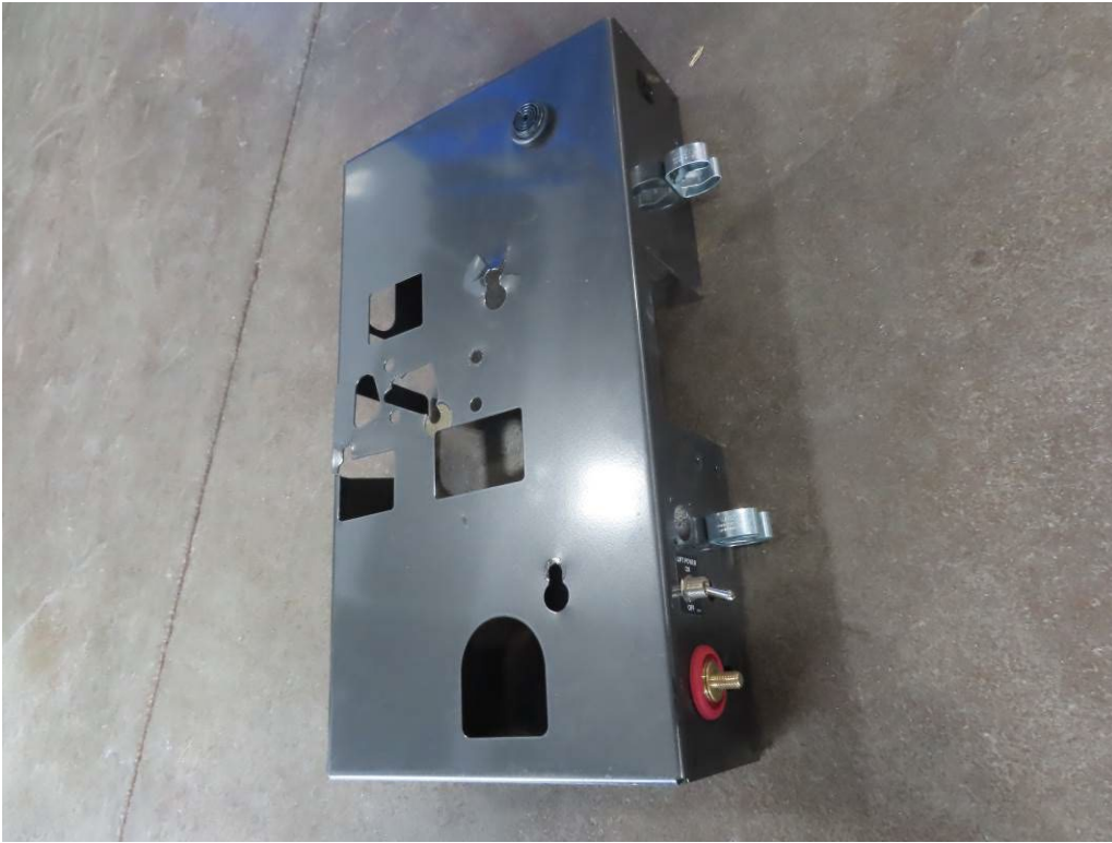
BROKEN COVER PANEL OF POWER BOX FOR ADA LIFT (2,521 TEST MILES)
