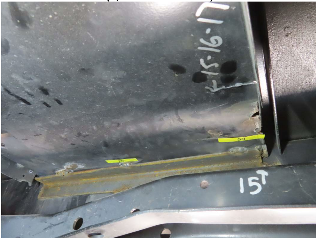
CRACKS #52 & 53 – CRACKS IN REAR HEATSHIELD ABOVE HORIZONTAL CROSSMEMBER (7,486 TEST MILES)
