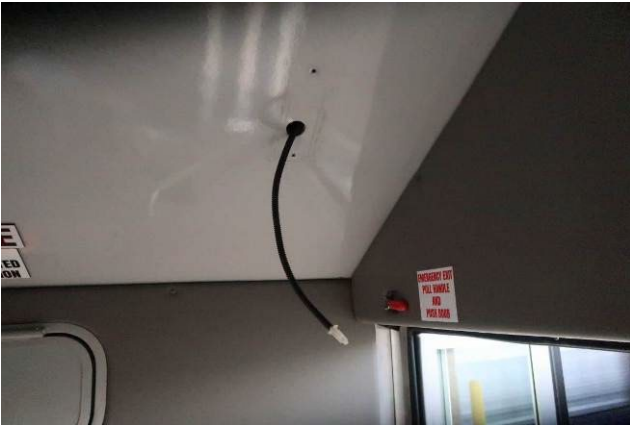
INTERIOR LIGHT OVER PASSENGER DOOR FELL DOWN (7,486 TEST MILES)
