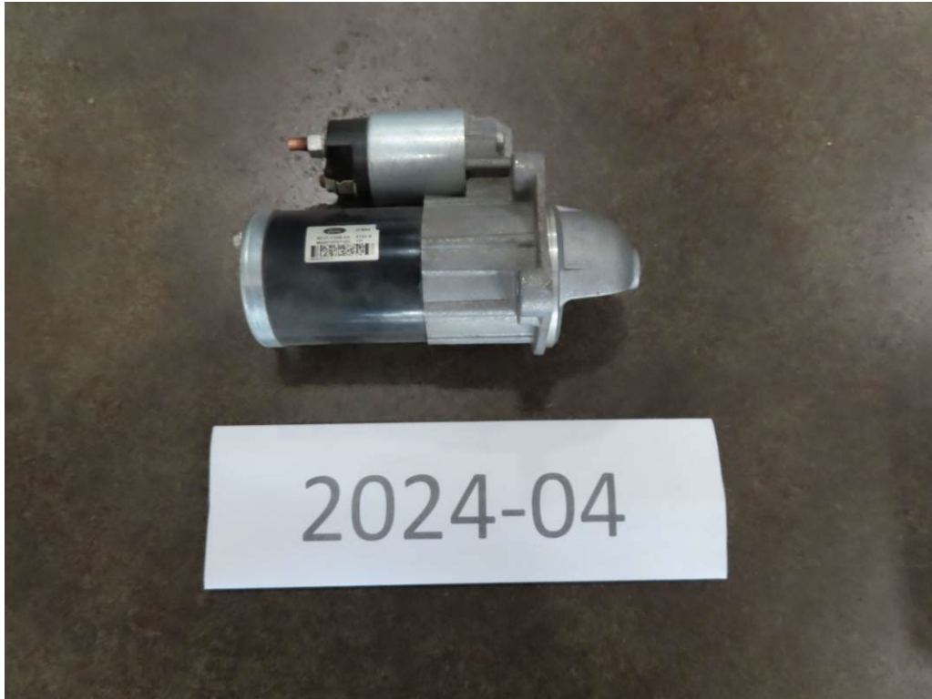
STARTER REMOVAL AND REPLACEMENT (0.33 LABOR HOURS)
