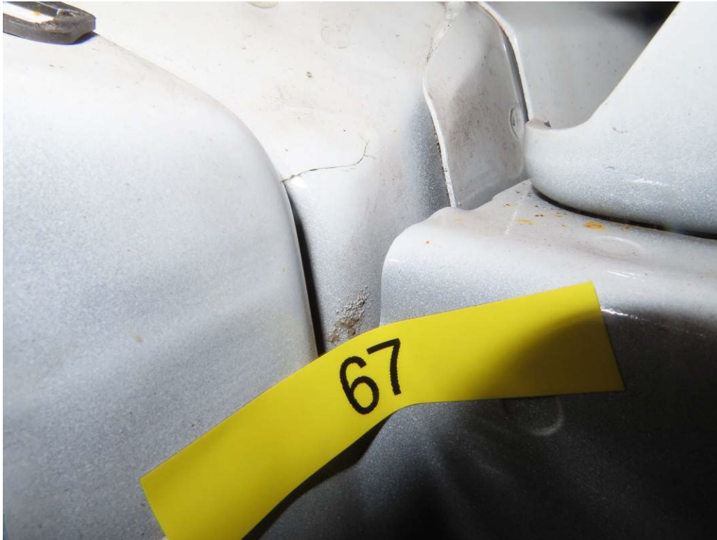
CRACK #67 – CURBSIDE BACKSIDE OF INNER FENDER UNDER CORNER OF WINDSHIELD (7,486 TEST MILES)
