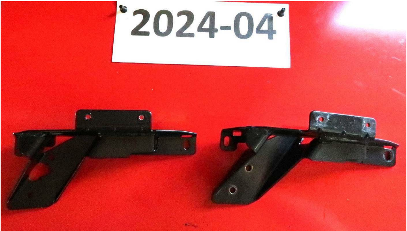
MODIFIED BRACKET FOR CURBSIDE FRONT MIRROR (LEFT) ORIGINAL BRACKET (RIGHT) (7,034 TEST MILES)
