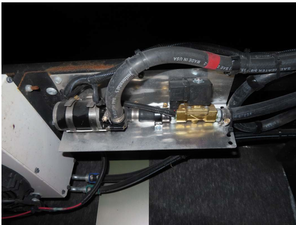
COOLANT PUMP ASSEMBLY REPLACED (1,123 TEST MILES)
