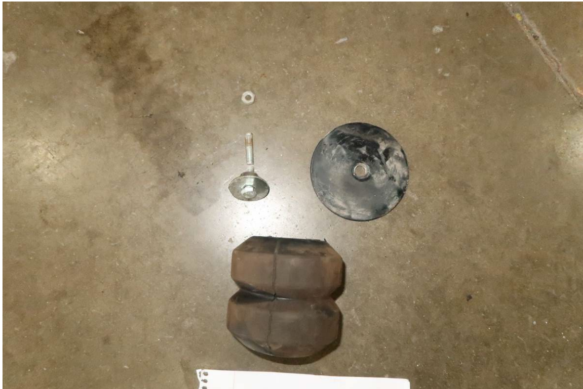
FRONT CURBSIDE BUMP STOP BROKE AND FELL OFF (4,781 TEST MILES)
