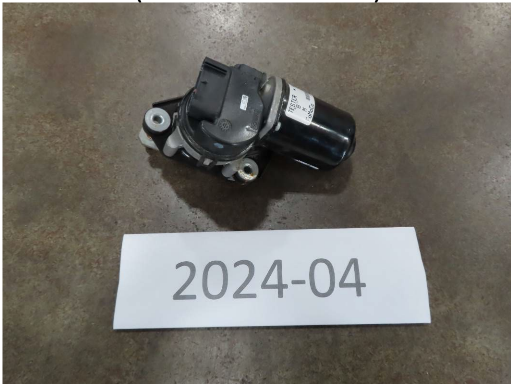
WIPER MOTOR REMOVAL AND REPLACEMENT (0.17 LABOR HOURS)
