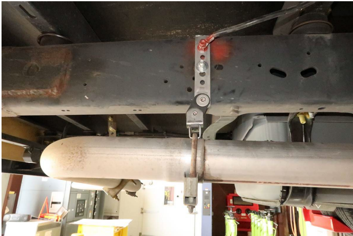
EXHAUST HANGER REPLACED (7,324 TEST MILES)
