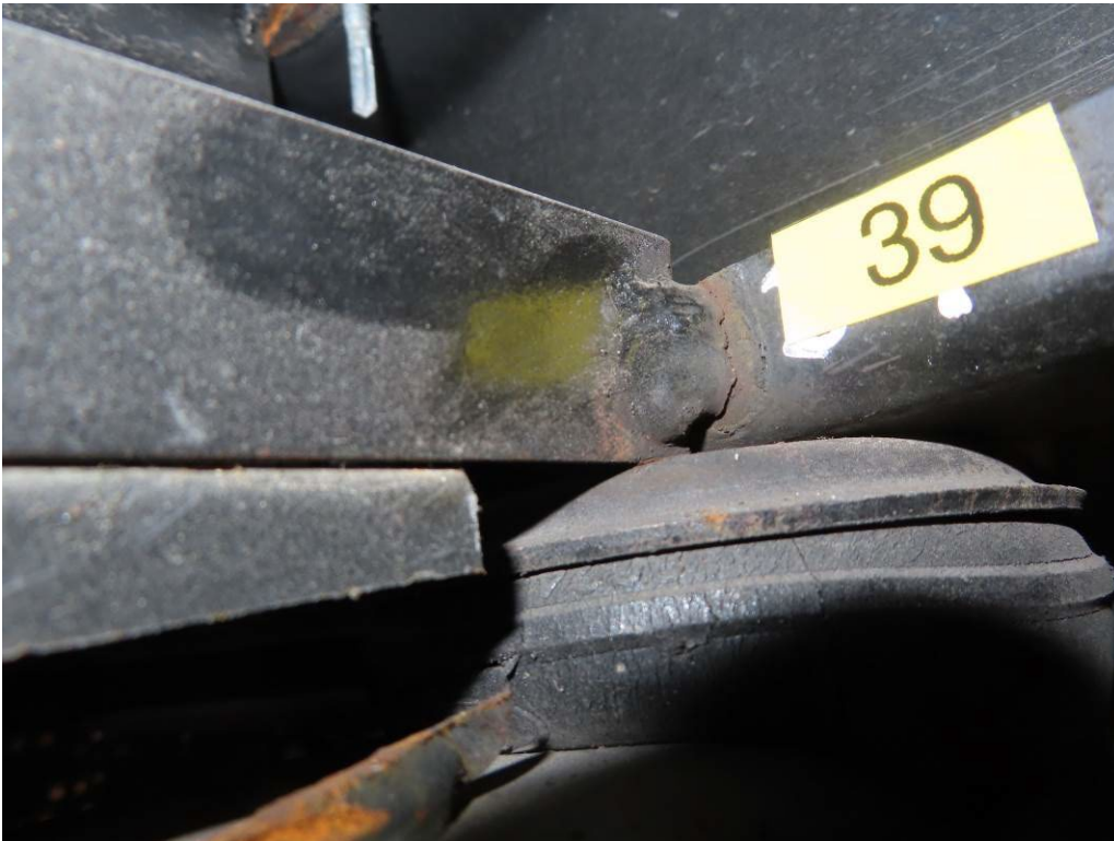
CRACK #39 – CRACK ON THE HEATSHIELD (6,207 TEST MILES)
