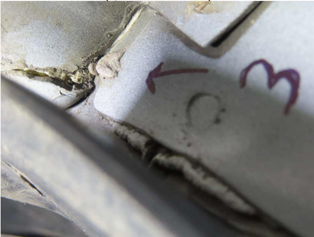
CRACK #3 – FRONT CURBSIDE INNER FENDER IS PULLING AWAY/CRACKED ON THE REAR LOWER SIDE (1,123 TEST MILES)
