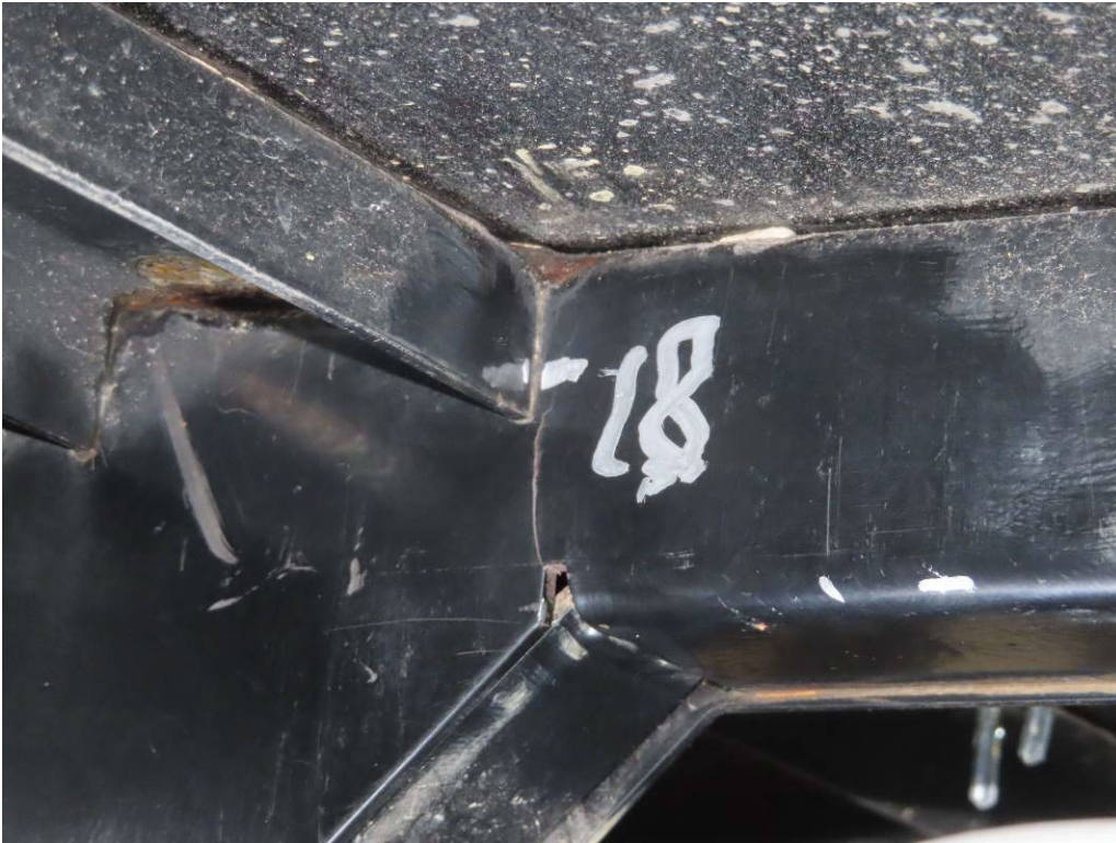
CRACK #18 – CURBSIDE CROSSBEAM WHERE CUT OUTS WERE MADE FOR FUEL TANK (1,123 TEST MILES)
