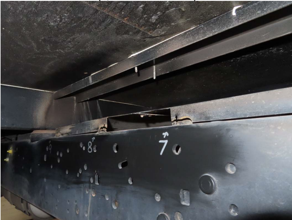
CRACKS #7, 8 & 9 – TOP OF THE CURBSIDE FRAME WHERE THE HEATSHIELD IS WELDED (1,123 TEST MILES)
