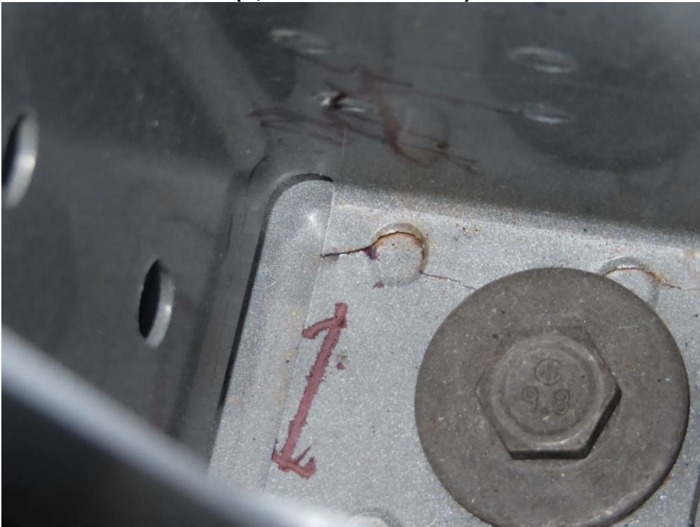
CRACK #1 – SPOT WELDS AROUND CORE SUPPORT, STREETSIDE (1,123 TEST MILES)
