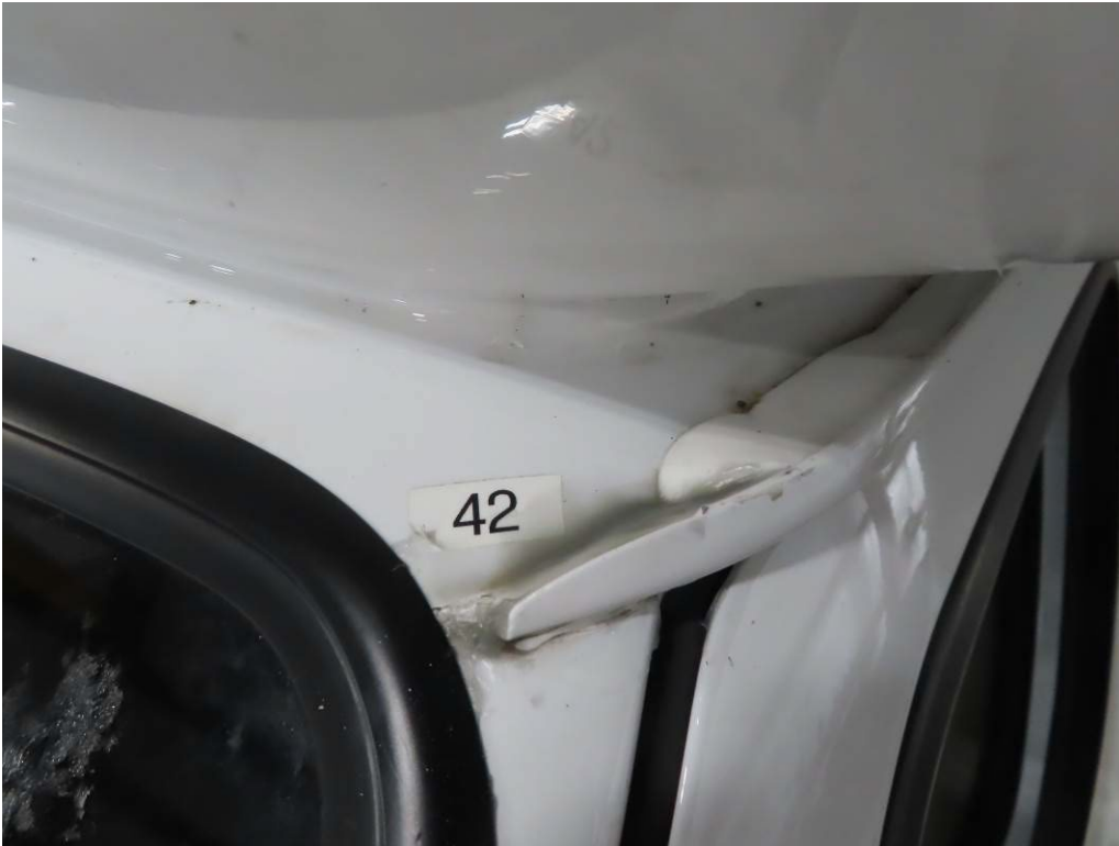
CRACK #42 – A CRACK IN THE STREETSIDE UPPER CORNER OF THE WINDSHIELD NEAR THE DRIP EDGE (6,207 TEST MILES)
