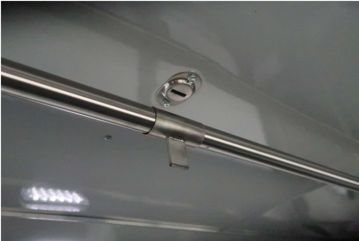
BROKEN WELD ON CURBSIDE GRAB HANDRAIL (7,034 TEST MILES)
