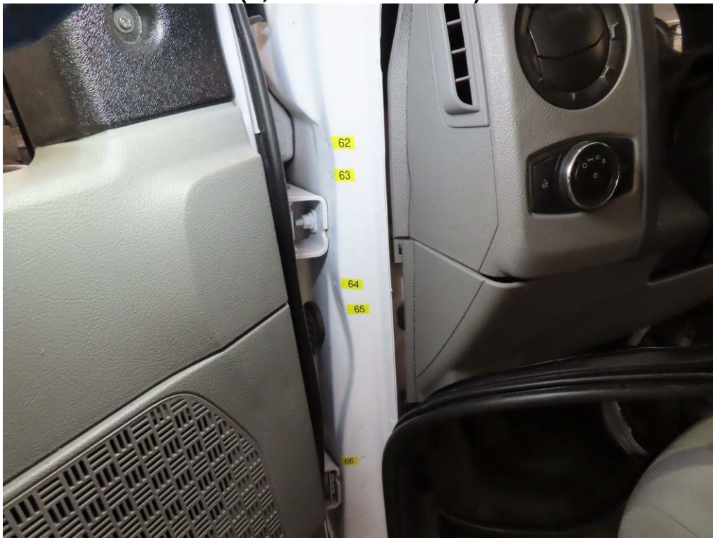
CRACKS #62, 63, 64 & 65 – LOCATION OF CRACKS IN DRIVER'S DOOR JAMB (7,486 TEST MILES)
