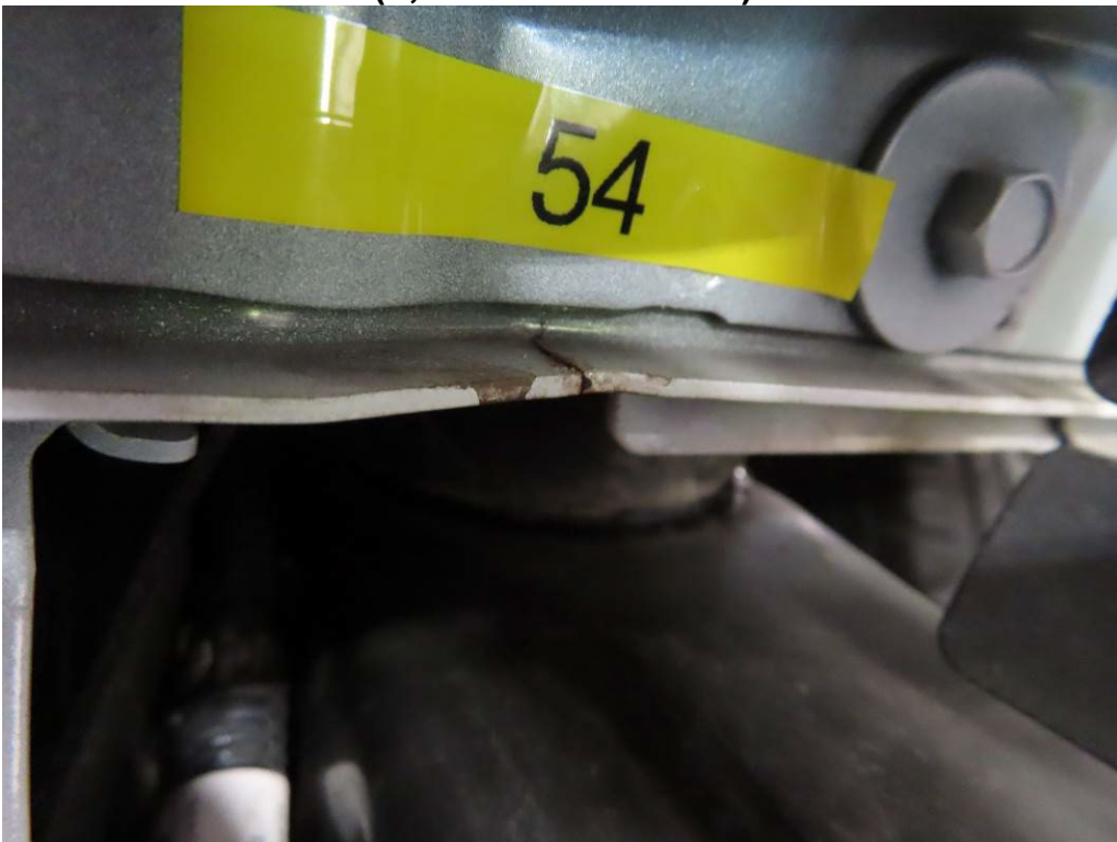
CRACK #54 – CRACK IN BODY BEHIND GRILLE IN FRONT OF THE A/C CONDENSER (7,486 TEST MILES)
