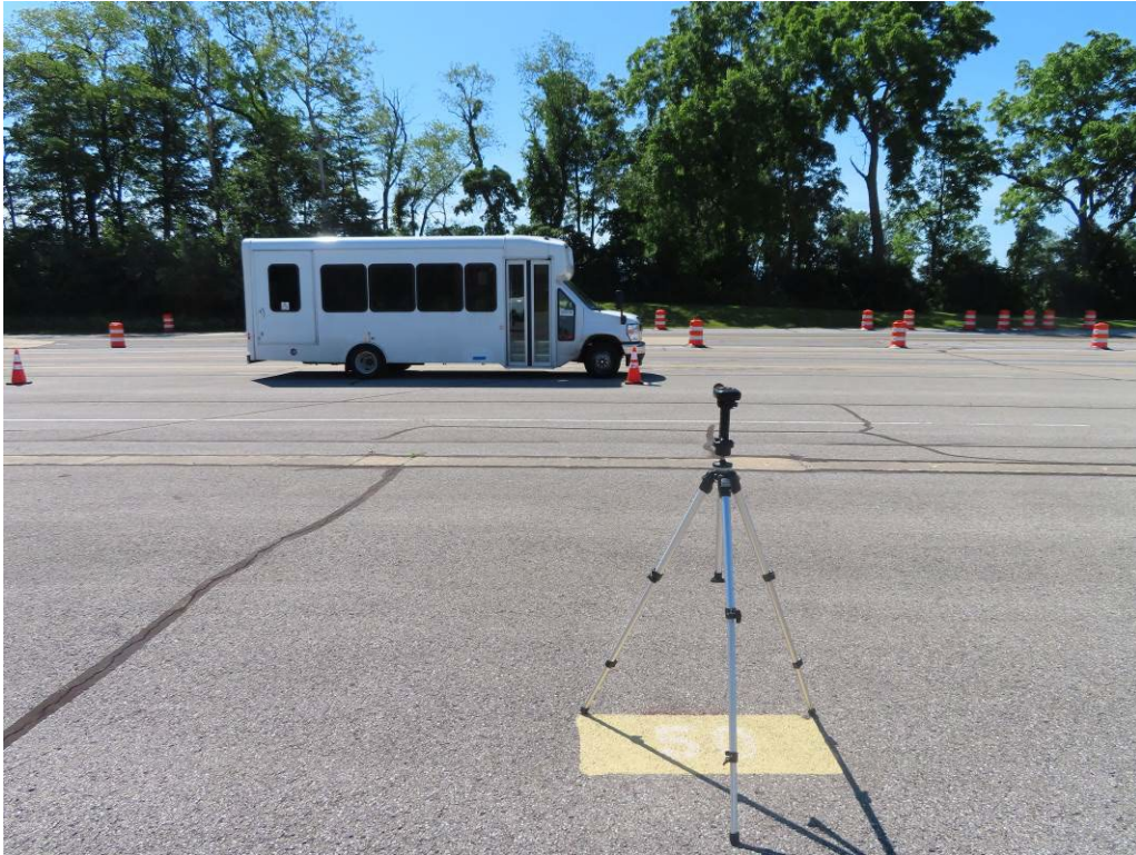
TEST BUS UNDERGOING EXTERIOR NOISE TESTING
