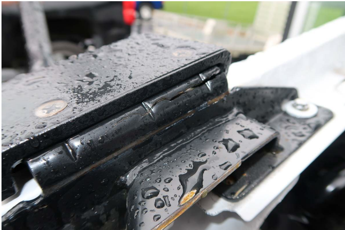
CURBSIDE FRONT MIRROR BRACKET IS CRACKED (4,183 TEST MILES)
