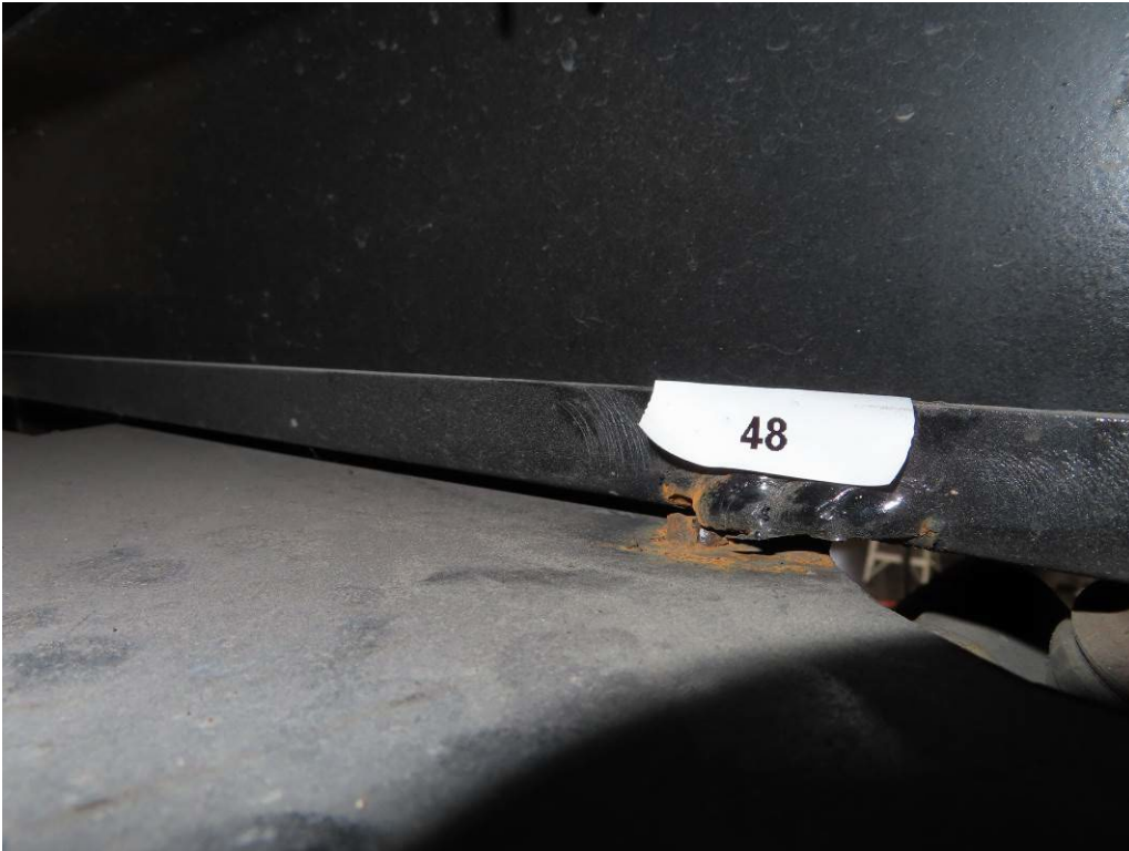
CRACK #48 – WELD ON THE HEATSHIELD ABOVE CURBSIDE FRAME RAIL INSIDE THE BODY MOUNT JUST FORWARD OF CRACK #27-2 (7,486 TEST MILES)
