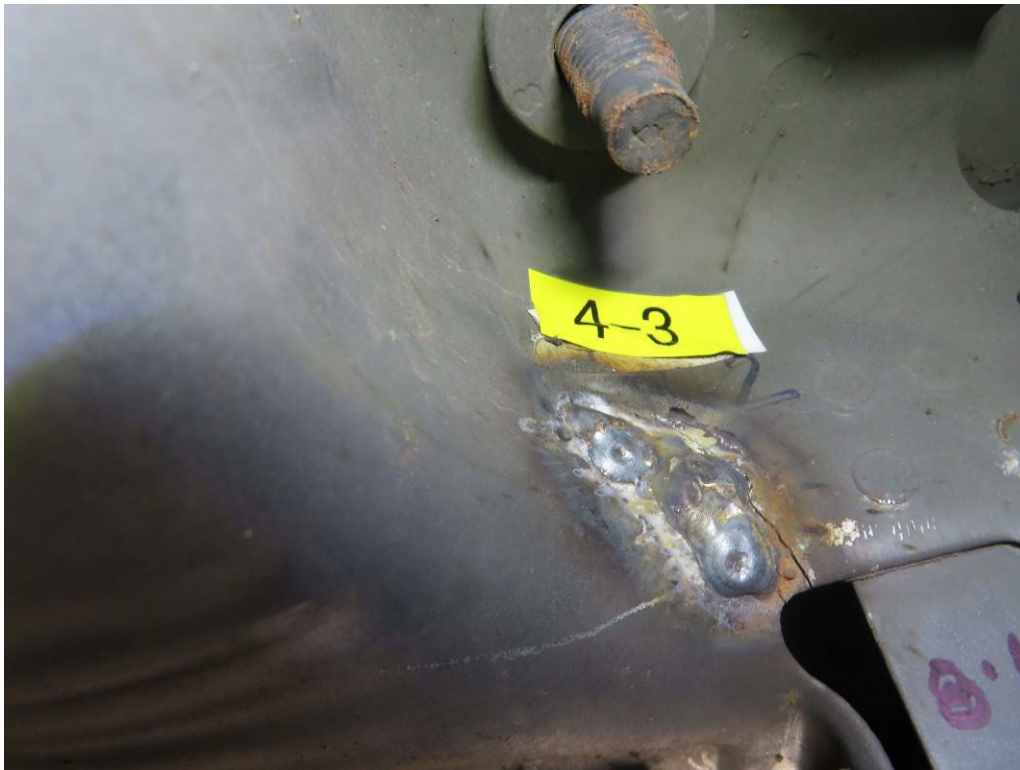
CRACK #4-3 – PREVIOUSLY WELDED CRACK IN BODY BELOW REAR LEFT DRIVER’S SEAT BOLT CRACKED AGAIN (7,486 TEST MILES)
