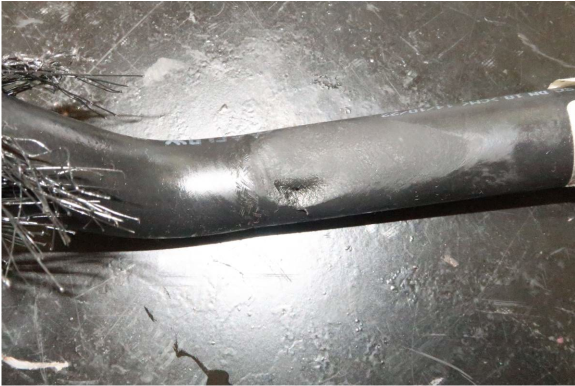
HOLE ON INTAKE HOSE OF POWER STEERING PUMP (6,118 TEST MILES)
