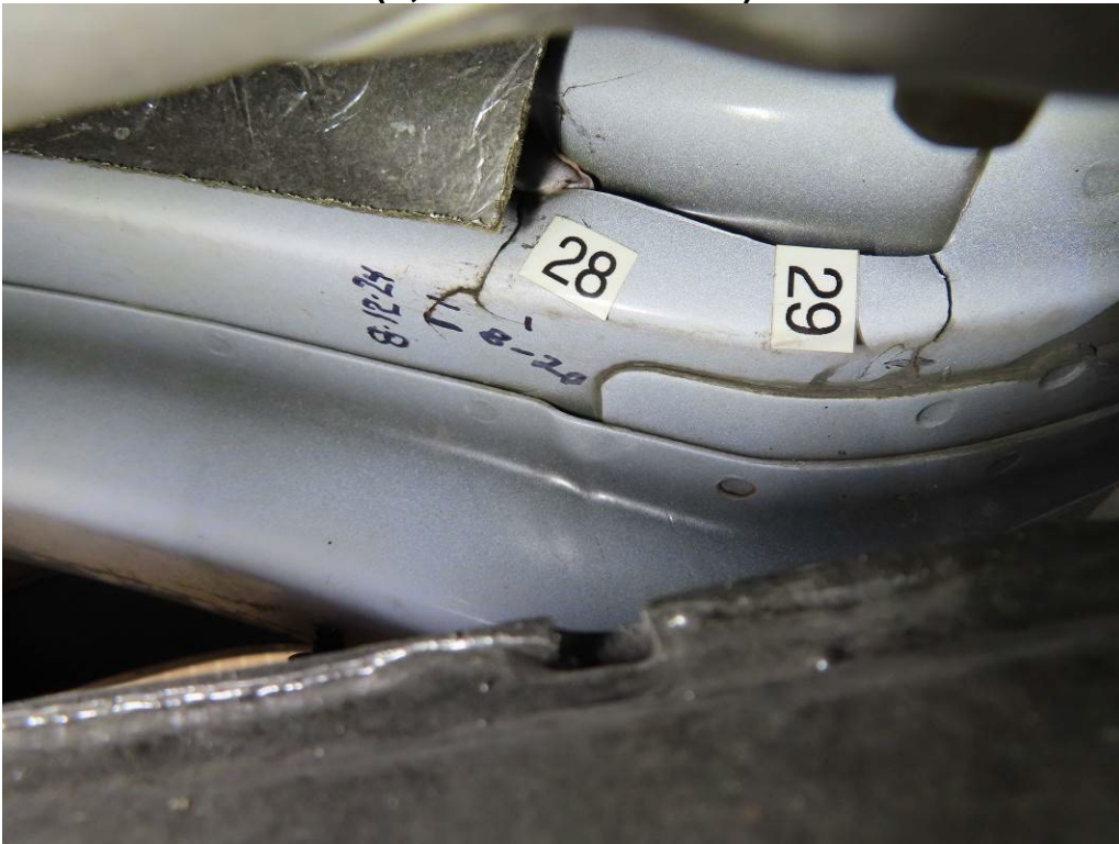
CRACKS #28 & 29 –ON THE BODY AT THE BACK OF THE CURBSIDE FRONT INNER FENDER ABOVE FRAME RAIL (7,486 TEST MILES)
