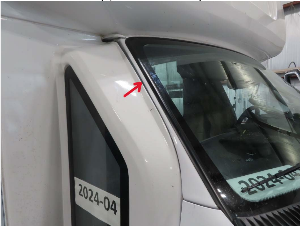
CAULKING IS SEPARATING BETWEEN SUPPORT POST AND WINDSHIELD (4,975 TEST MILES)
