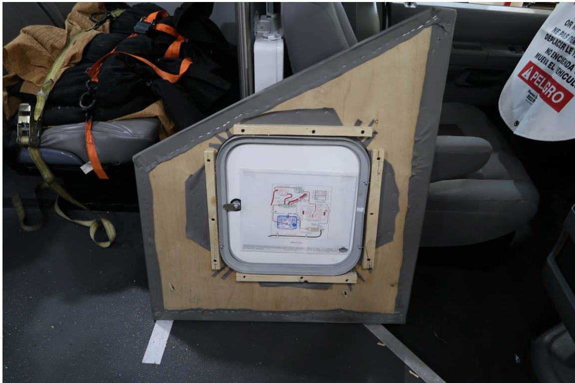
ELECTRICAL SYSTEM COVER PANEL ABOVE DRIVER FELL DOWN (4,183 TEST MILES)
