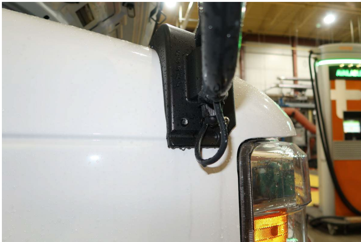
SCREW FELL OUT OF CURBSIDE MIRROR (300 TEST MILES)
