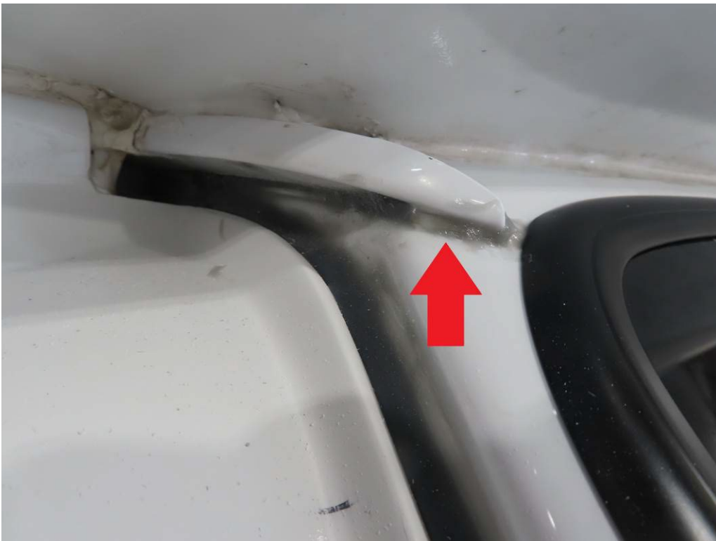
CRACK #33 AT CURBSIDE TOP OF WINDSHIELD REPAIRED WITH EPOXY AND SILICONE (4,975 TEST MILES)
