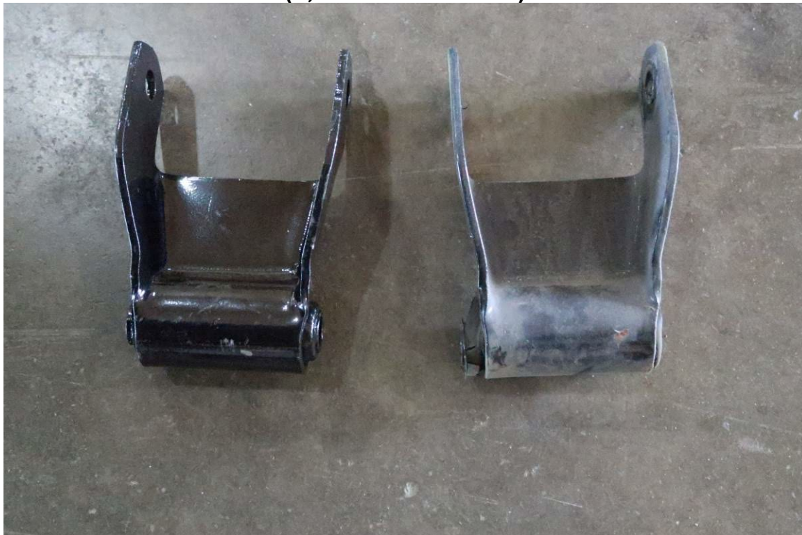
REPLACEMENT SPRING SHACKLE (LEFT) / WORN STREETSIDE REAR SPRING SHACKLE (RIGHT) (3,551 TEST MILES)
