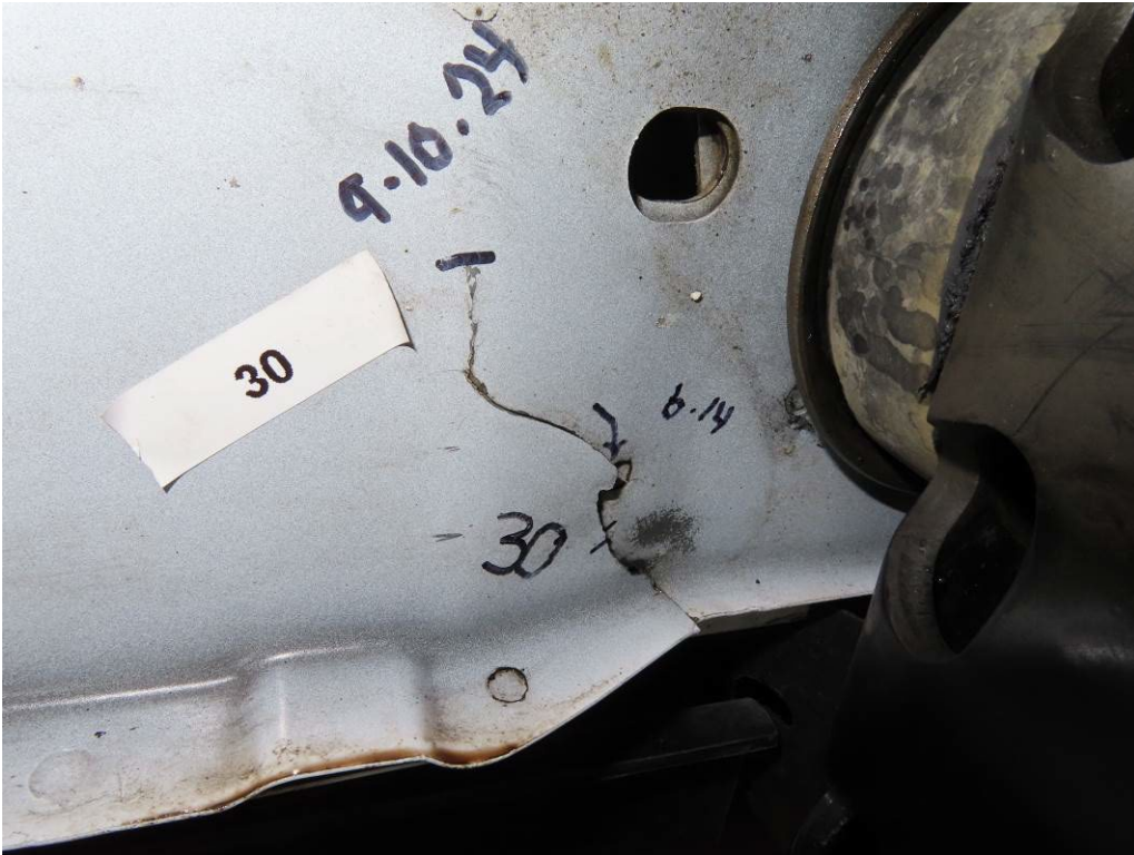
CRACK #30 – STREETSIDE BODY ABOVE THE FRAME RAIL ADJACENT TO THE FORWARDMOST BODY MOUNT BUSHING (7,486 TEST MILES)
