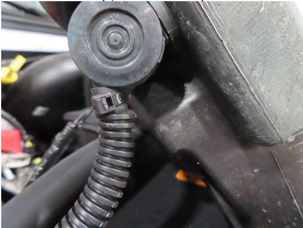
REPAIRED BROKEN HOSE ON WASHER PUMP (2,521 TEST MILES)
