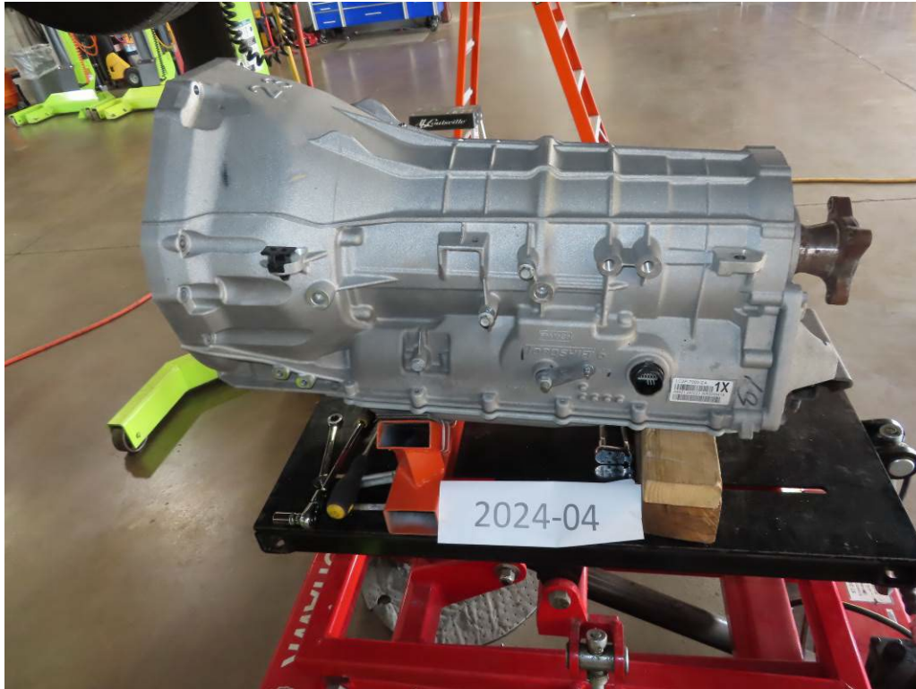
TRANSMISSION REMOVAL AND REPLACEMENT (7.00 LABOR HOURS)
