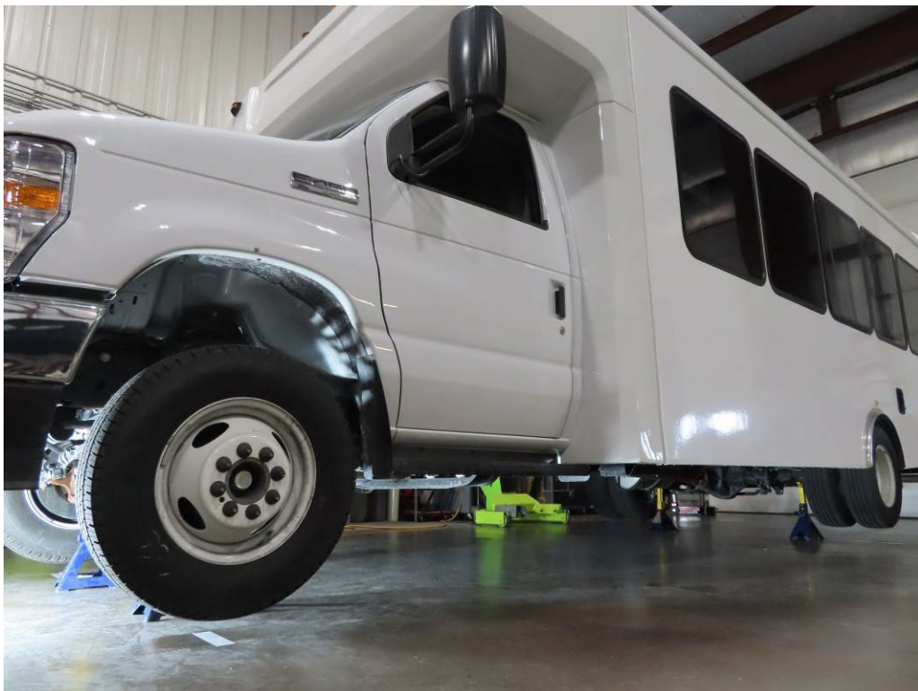
JACK STANDS IN PLACE – FRONT AND REAR
