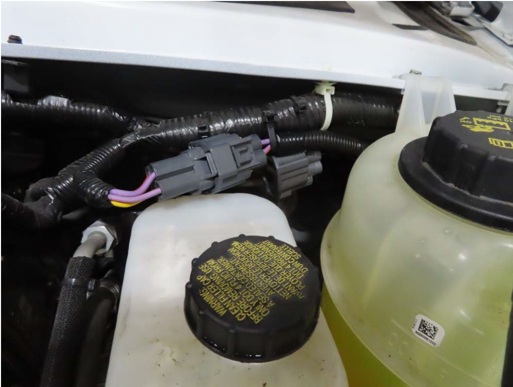
JUMPER HARNESS FOR HIGH IDLE INSTALLED (4,579 TEST MILES)
