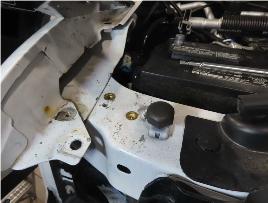
HOLES DRILLED IN CORE SUPPORT AREA AND NUTSERTS ADDED FOR MIRROR MOUNTING (4,975 TEST MILES)
