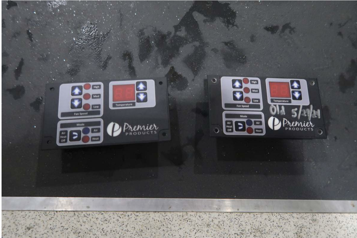
DEFECTIVE CONTROL BOARD FOR REAR A/C REPLACED (4,183 TEST MILES)
